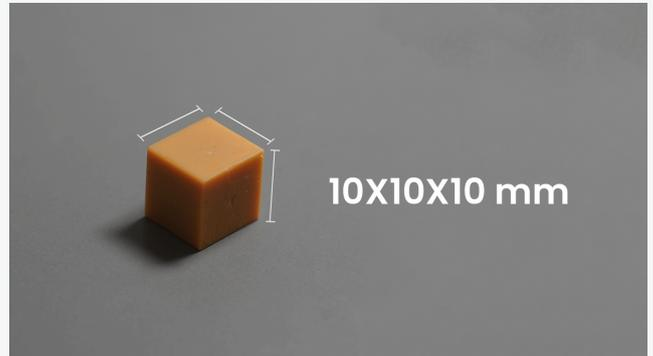
Measure each length of the block in the X and Y directions. If it is less than 10mm, slightly increase the Exposure Time by 0.5-1 second each time.
